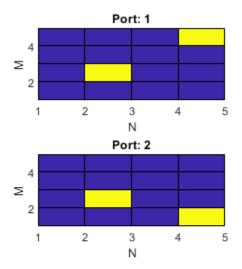
Create a 3D received grid to extract resource elements. Extract resource elements from the received grid. Show the locations of these extracted resource elements. Addressed resource element locations contain 1.
