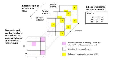
The following diagram shows the extraction process for a 4D channel estimate grid, grid, with NRxAnts = 3 and P= 2. In this case, P is the number for antenna ports. The 4D resource grid consists
