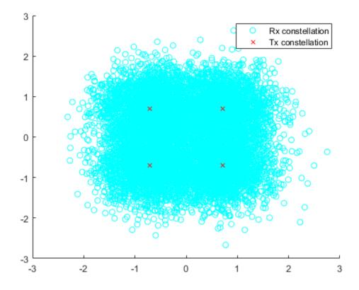
Demodulate the symbols and turbo decode soft bits. Compare the transmitted and recovered bits.
