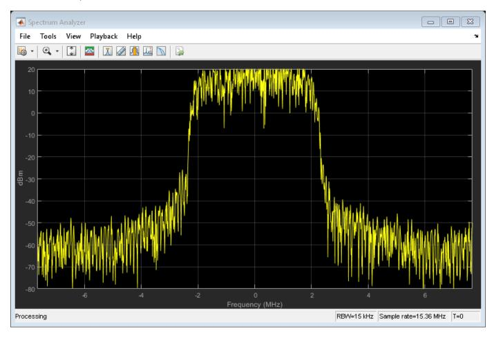
waveform = umtsDownlinkWaveformGenerator(frcStruct); saScope = dsp.SpectrumAnalyzer('SampleRate', 3.84e6\*frcStruct.OversamplingRatio); saScope(waveform);
