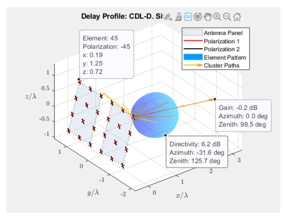
Visualize and explore channel characteristics at the receiver end. To customize the receive antenna array, use the ReceiveAntennaArray property of the lte3DChannel System object. Then, display the channel characteristics at the receiver end by calling the displayChannel function with the 'LinkEnd', 'Rx' name-value pair argument.
