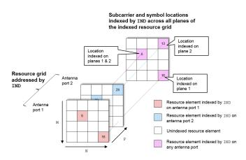
Resource elements are extracted from grid at the symbol and subcarrier locations. The following diagrams illustrate the resource element extraction from a 3D received grid, grid, with NRxAnts = 3.
