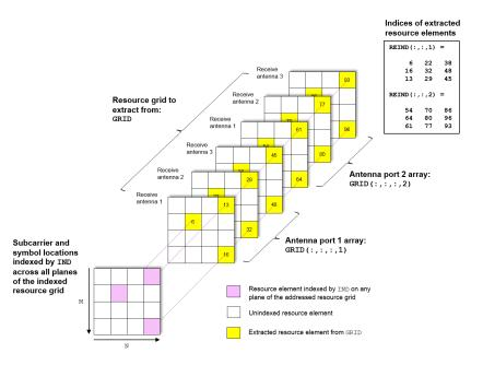
of *P M*-by-*N*-by-*NRxAnts* arrays, each associated with an antenna port. Resource elements are extracted from all planes within these arrays.
