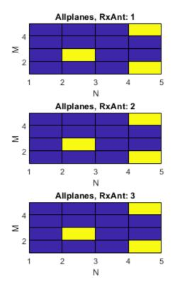
Create a 4D channel estimate grid to extract resource elements. Extract resource elements from the channel estimate grid. Show the locations of these extracted resource elements. Addressed resource element locations contain 1.
