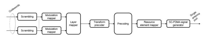
For PSSCH, the input codeword length is  $M_{\text{bits}} = N_{\text{RE}} \times N_{\text{bps}}$ , where  $N_{\text{bps}}$  is the number of bits per symbol. PSSCH modulation is either QPSK (2 bits per symbol) or 16 QAM (4 bits per symbol).
